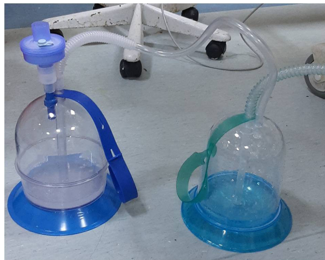
Figure 2. The combined use of traditional drainage bottles to prevent virus spread. The first bottle is connected to a second bottle with a hose. One bottle contains 70% ethyl alcohol and the other bottle contains 10% concentration NaOCl. A viral/bacterial filter has also been added to the air cannula of the last bottle.
