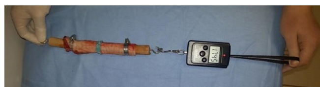
Figure 2. Scaling the tensile strength by an electronic spring scale.
